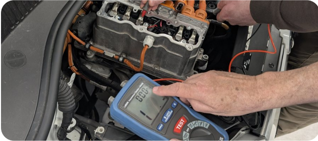
Electrical safety and insulation checks
